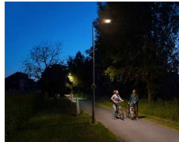
Column lighting should include motion detectors where possible to allow variable light levels on footpaths and cycleways (ref: Schröder)
